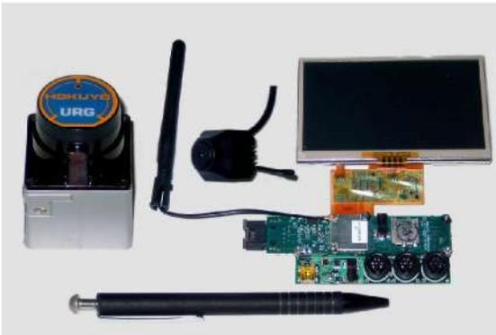
Fig. 13: FROM THE LEFT TO THE RIGHT A HOKUYO URG-04LX LASER RANGE-FINDER, A WIRELESS VISORTECH GP-811T CAMERA AND GUMSTIX VERDEX XL6P COMPUTER WITH 802.11 (G) WIRELESS COMMUNICATION MODULE ARE SHOWN. THE DISPLAY IS DETACHABLE AND IS NOT NEEDED DURING THE FLIGHT.
