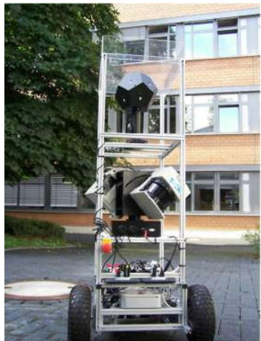
Fig. 1: FIRST EVALUATION PLATFORM OF THE UGAV. THE GROUND PLATFORM IS BUILT OF A VOLKSBOT RT3 WHICH IS EQUIPPED WITH BATTERIES, VISION SENSORS, 3D LASER SCANNER, CONTROL COMPUTERS AND A LANDING PLATFORM ON TOP FOR THE QUADROTOR.
